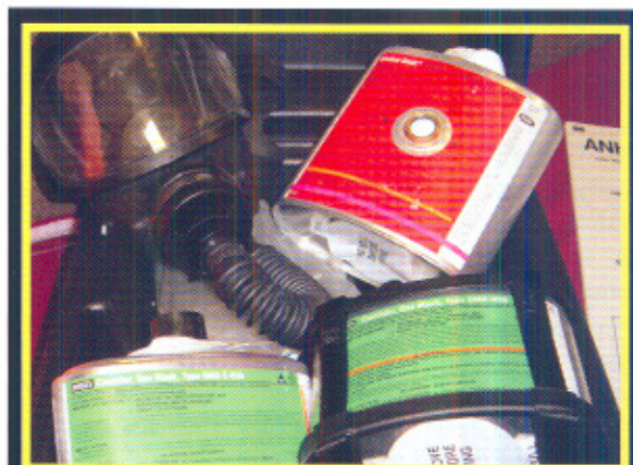
A full-face respirator must be worn when ammonia concentrations in the air reach 300 ppm.
