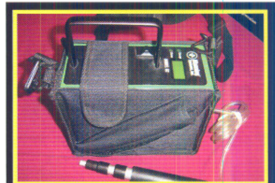
Portable sampling units can provide instant readings using a hand-held wand.
